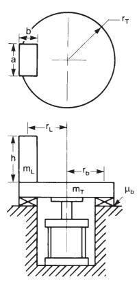
Acceleration =  $\alpha$ The index table rotates in a horizontal plane, with a rectangular load.
