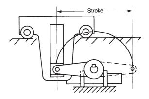
The harmonic motion linkage shown is a compact, low cost method of producing linear motion with smooth acceleration and deceleration. This property permits the cycle times of applications such as transfer lines to be optimized.
