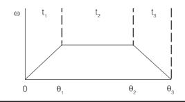
$$t_{1} = 2 \quad \frac{\theta_{1} - 0}{\omega} = 2 \left(\frac{10^{\circ}}{\omega}\right) \frac{\pi}{180^{\circ}} = \frac{(0.35)}{\omega}$$
