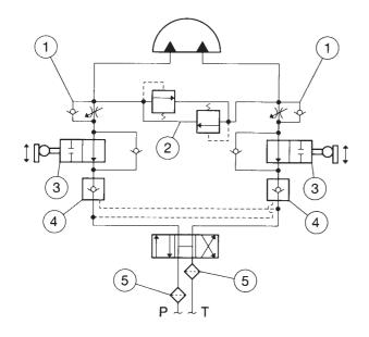
As with most standard hydraulic circuits, rotary actuator applications should have filtration to provide a continuous cleanliness rating in accordance with the ISO 17/14 fluid classification. Filters (5) should be fitted and maintained to ensure this minimum level.
