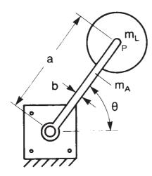
The load is rotated through a vertical plane. Load torque M, is positive or negative, depending on position and direction of rotation.
