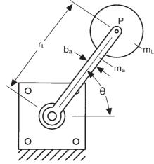
Paper roll, 70 kg, pivoted at P. Lever arm, 6kg (1.5m long, 0.3m wide ).
