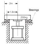
Platform mass = 200kg Bearing radius = 1.8m Angular acceleration  $\alpha$  = 2 rad/sec<sup>2</sup> Bearing coefficient of friction  $\mu$  = 0.25 Rotational mass moment of inertia J<sub>m</sub> = 400kgm<sup>2</sup>
